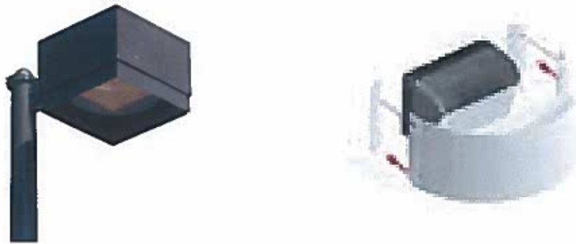
Figure B: Mounting height or proximity to property lines may cause the luminous elements of a light fixture to need additional shielding. Above are two examples of shielding.
