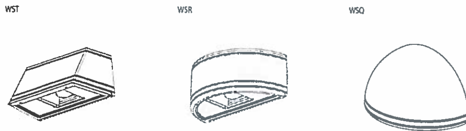
Figure L: Samples of acceptable wall packs
